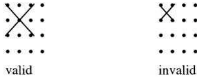
Fig. 2. Wires may only cross at end points, not in the middle of segments
