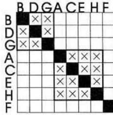
Fig. 2. The same DSM in Figure 1 but after reordered. The DSM can be cleanly clustered as ((B,D,G)(A,C,E,H),(F)).
